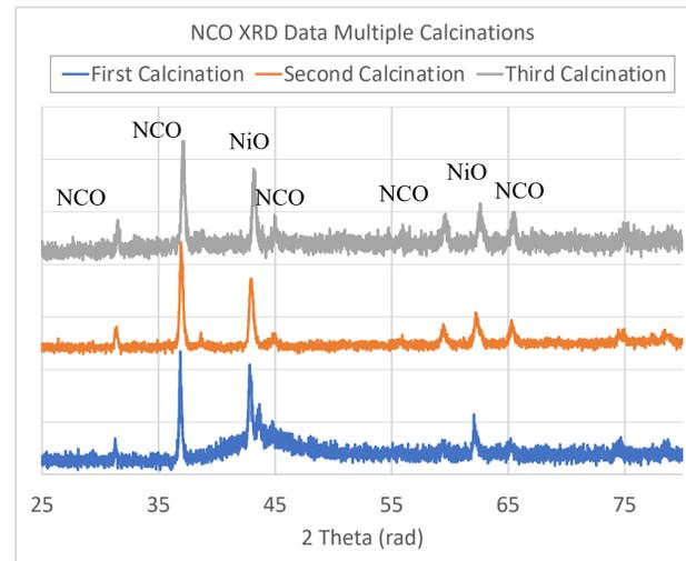
Figure 4 – Sample of NiO and  $\text{Co}_3\text{O}_4$  mixed in a Ni/Co molar ratio of 1:2
