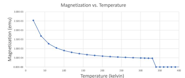
Figure 9 – Field cooled at 5T – sudden drop at 340K is from dislodging of the sample
