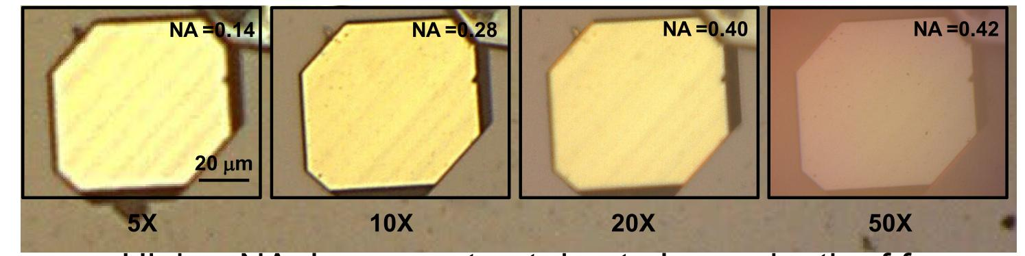
Higher NA, lower contrast due to lower depth of focus
