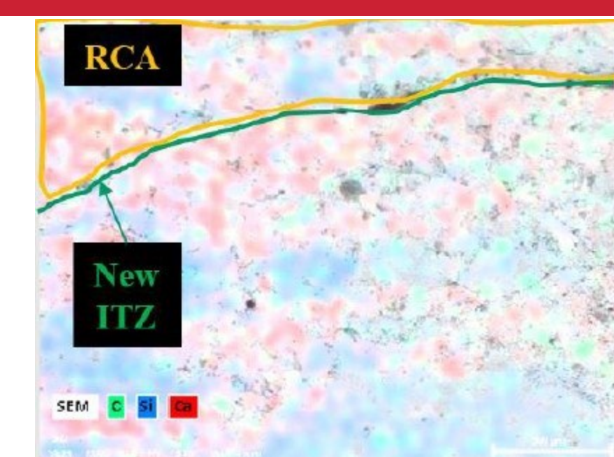
SEM figure of 5% addition of Biochar for improved aggregate-cement paste bonding
