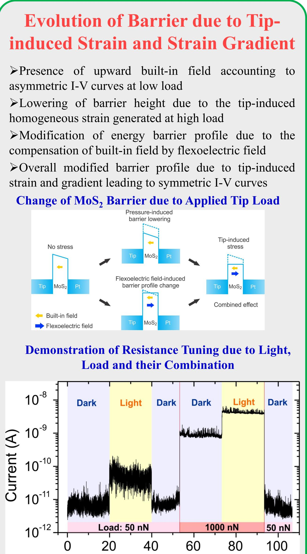
Enhanced MoS<sub>2</sub> conductivity due to tip load or light Combined excitation approach adds to further enhancement (~ 1 order of magnitude) of conductivity
