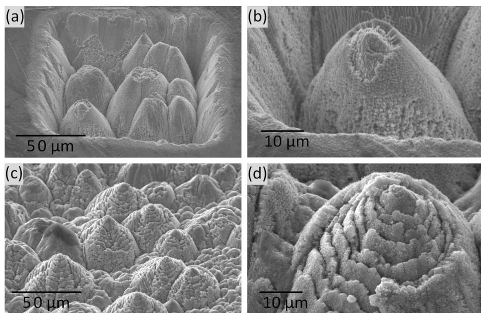
**Fig. 4.** SEM images of pyramids formed using the following parameters: parts (a) and (b) stationary ablation with the square flat-top profile using 20,000 pulses at  $0.12 \text{ J/cm}^2$ , after cleaning in an ultrasonic bath. Parts (c) and (d) rastering Gaussian focused pulses with 30,000 pulses/area at  $0.248 \text{ J/cm}^2$ , after cleaning in an ultrasonic bath.
