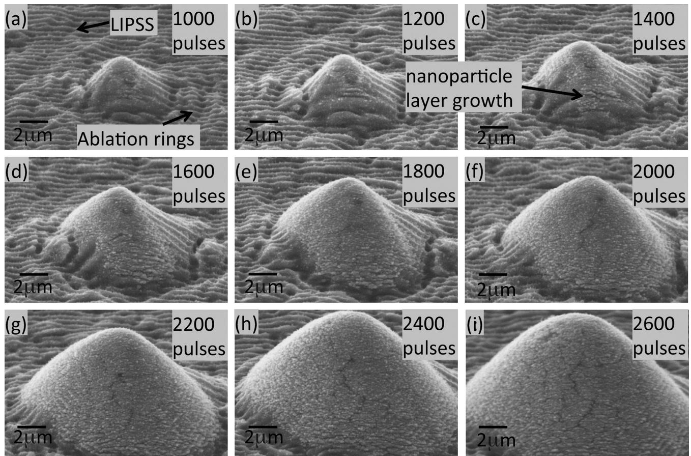
**Fig. 1.** (multimedia online: media 1). SEM images of stepped NC-pyramid growth from the stop-motion SEM analysis of nickel imaged at  $45^\circ$  after the specified number of pulses. Part (a) represents the end of the first phase. Parts (b)–(i) represent the second phase. These images represent single frames of media 1.
