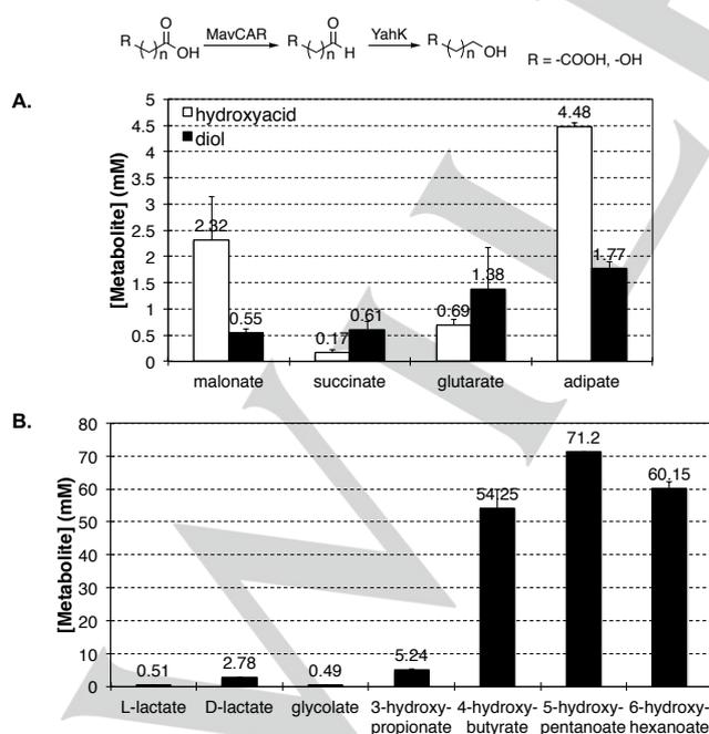
**Figure 5.** Reduction of short-chain carboxylates using *E. coli* cells expressing MavCAR and YahK. The x-axis represents the substrates spiked in the culture media. (A) Dicarboxylic acid substrates. (B) Hydroxyacid substrates. Cells were cultured in media (pH 7.0) containing 100 mM of indicated carboxylate. Data are the average of three measurements with standard deviation.
