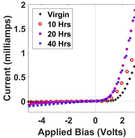
Fig. 2. (Color online) Current vs voltage curves of a  $a\text{-B}_{10}\text{C}_{2+x}\text{H}_y$  to silicon heterojunction diode following 0,  $2.7 \times 10^8$ ,  $5.4 \times 10^8$ , and  $10.8 \times 10^8$  neutrons/cm<sup>2</sup> exposure (0, 10, 20, and 40 h of exposure to neutron irradiation, under our experimental conditions).
