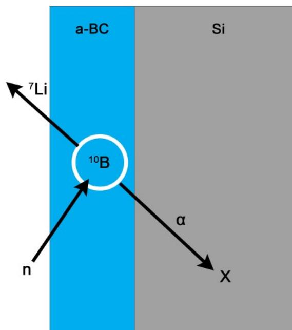
FIG. 1. (Color online) Depiction of neutron capture by a  ${}^{10}\text{B}$  isotope resulting in fragmentation into a  ${}^7\text{Li}$  and  $\alpha$  particle pair with kinetic energy resulting in translation away from the capture site (not to scale). Unless ion translation is parallel to the interface, one ion will exit the  $a\text{-B}_{10}\text{C}_{2+x}\text{H}_y$  film, and one will implant within the Si substrate, as represented by the “x.”
