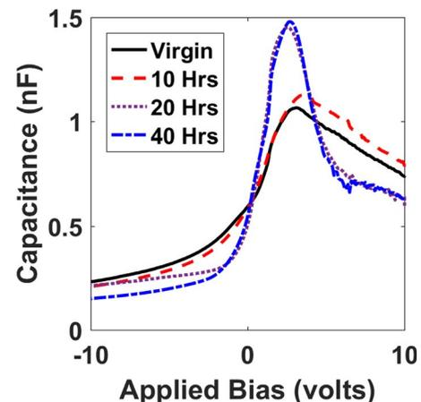
Fig. 3. (Color online) Capacitance vs voltage  $C(V)$  curves taken at 100 kHz of  $a\text{-B}_{10}\text{C}_{2+x}\text{H}_y/\text{Si}$  p-n heterojunction device after 0,  $2.7 \times 10^8$ ,  $5.4 \times 10^8$ , and  $10.8 \times 10^8$  neutrons/cm<sup>2</sup> exposure (0, 10, 20, and 40 h of exposure to neutron irradiation, under our experimental conditions).
