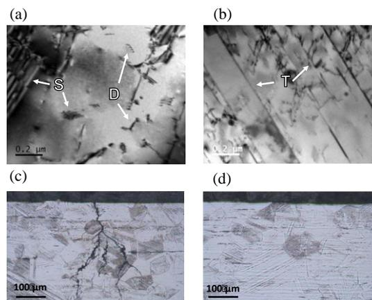
Fig. 1. (a)-(b) TEM images of near-surface microstructures of ODS 304 steels after LSP. S: stacking fault; D: dislocation; T: deformation twin. (c)-(d) Optical micrograph of the cross-section microstructures after SCC test of 72 hours: c) untreated 304 steels; d) LSP-treated 304 steels.
