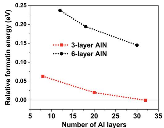
**Figure 3.** DFT calculations of the relative formation energy of Al/AlN with AlN in zinc blende phase compared to with AlN in wurtzite phase. Positive energy implies wz-AlN is more stable than zb-AlN.
