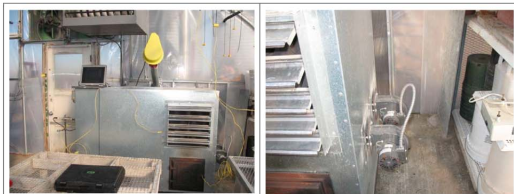
Figure 4. Biomass pellet burner (left) and combustion fans on right.
