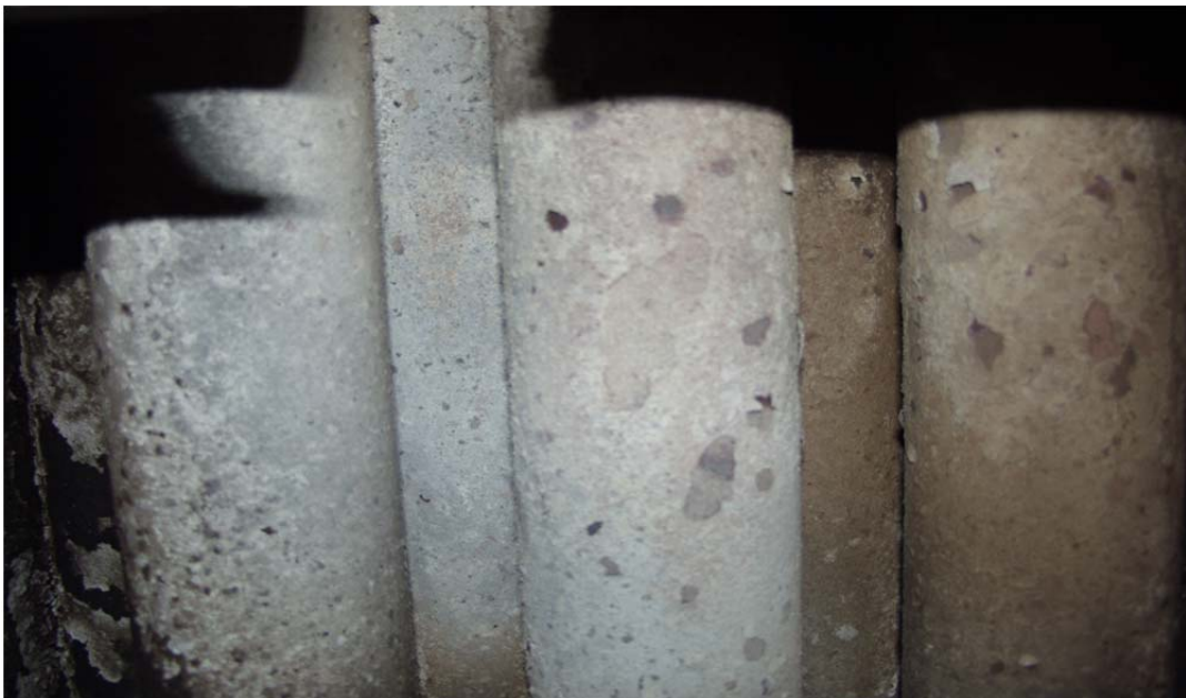
Figure 3.7. Fouling of Heat Exchanger Pipes.
