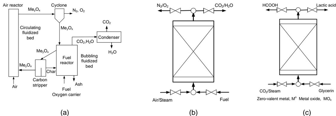
**Figure 1.** Reactor configurations for CLT: (a) Schematic of the CLC system, (b) Periodically operated CLT in packed bed system; (c) CO<sub>2</sub> conversion to formic acid in periodically operated CLT in packed bed system.
