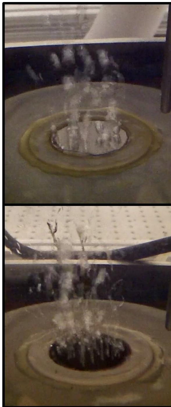
Fig. 6 Onset of boiling nucleation for both heat transfer surfaces: Top – polished sample, 13 \text{ }^\circ\text{C} superheat and 3 \text{ W/cm}^2 , Bottom – processed sample, 7.7 \text{ }^\circ\text{C} and 2 \text{ W/cm}^2
