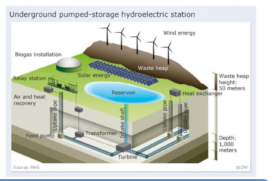
An UPHES facility has the same operating principle as PHES system: two reservoirs with a large hydraulic head between them. The only major difference between the two designs is the locations of their respective reservoirs. In conventional PHES, suitable geological formations must be identified to build the facility. However, UPHES facilities have been designed with the upper reservoir at ground level and the lower reservoir deep below the earth's surface [2].
