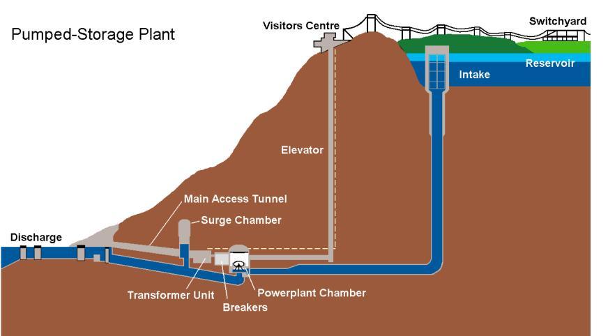
PHES is the most mature and largest storage technique available and consists of two large reservoirs located at different elevations and a number of pump/turbine units. During off-peak electrical demand, water is pumped from the lower reservoir to the higher reservoir where it is stored until it is needed. Once required the water in the upper reservoir is released through the turbines, which are connected to generators that produce electricity [2].
