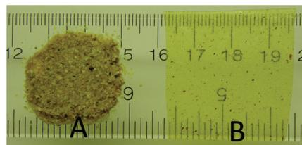
**Figure 9.** Digital image of DDGS without modification (A) and transparent thermoplastic film (B) developed from the cyanoethylated DDGS.
