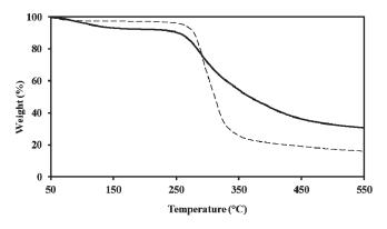
Figure 7. Comparison of the thermogravimetric curves for unmodified DDGS and cyanoethylated oil-and-zein-free DDGS with 42% weight gain.
