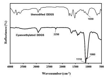
Figure 5. Infrared spectrum of unmodified DDGS and cyanoethylated DDGS with 42% weight gain.
