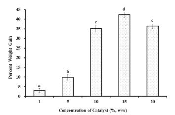
Figure 3. Effect of concentration of sodium hydroxide on percent weight gain of DDGS obtained after cyanoethylation. The cyanoethylation was carried out at 40  $^{\circ}$ C for 120 min with an acrylonitrile to oil-and-zein-free DDGS ratio of 5:1. Data points with the same letters indicate that they were not statistically different from each other.
