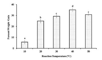
**Figure 2.** Effect of reaction temperature on percent weight gain of cyanoethylated DDGS. The cyanoethylation was carried out for 120 min with an acrylonitrile to DDGS ratio of 5:1 and a sodium hydroxide concentration of 10%. Data points with the same letters indicate that they were not statistically different from each other.
