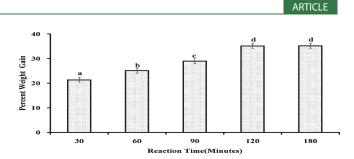
Figure 1. Effect of reaction time on percent weight gain of product obtained after cyanoethylation. The cyanoethylation was carried out at a temperature of 40  $^{\circ}$ C, an acrylonitrile DDGS ratio of 5:1, and a sodium hydroxide concentration of 10%. Data points with the same letters indicate that they were not statistically different from each other.
