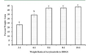
**Figure 4.** Effect of weight ratio of acrylonitrile to DDGS on the percent weight gain. The cyanoethylation was carried out at 40 °C for 120 min with a sodium hydroxide concentration of 15%. Data points with the same letters indicate that they were not statistically different from each other.
