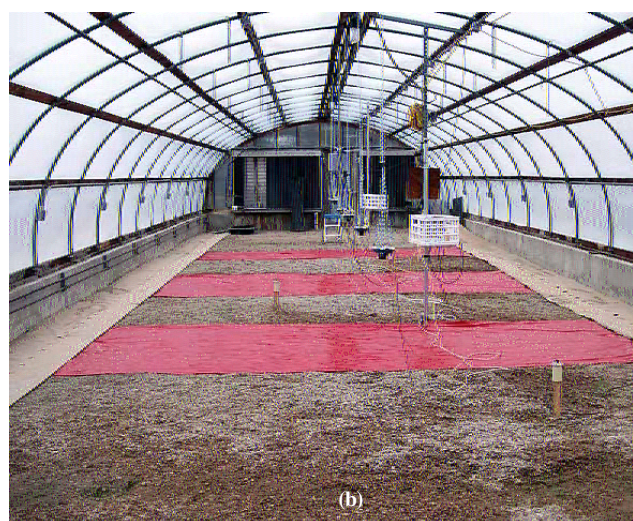
Figure 1. Reflective mulch and surface temperature study with (a) 6-mil white plastic and (b) 1-mil red plastic (Rotation of black and dark olive plastic mulches are not shown).
