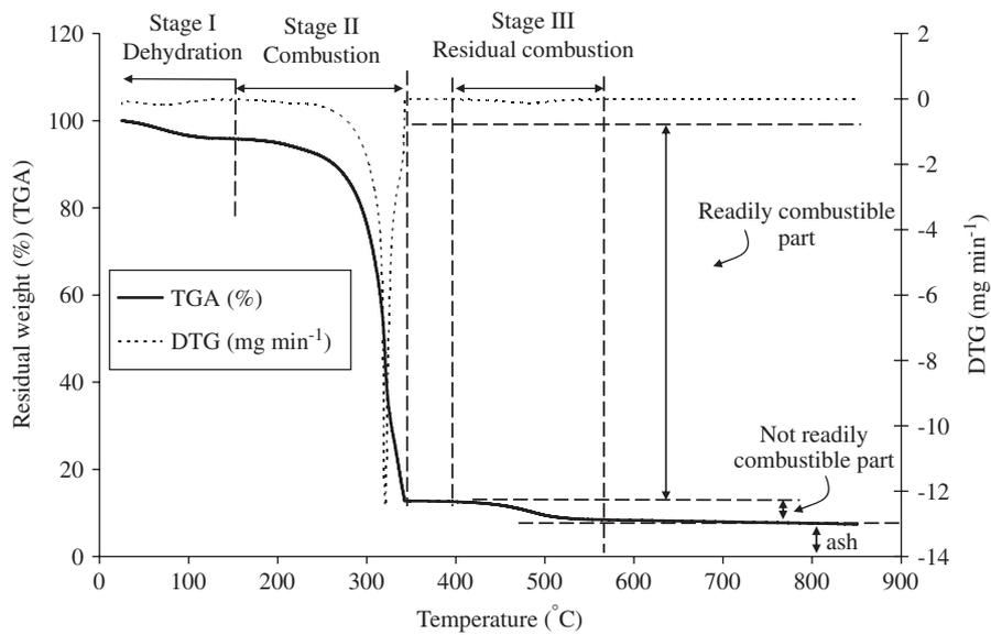
Fig. 4 – Typical TGA plot of corn stover in an air atmosphere.
