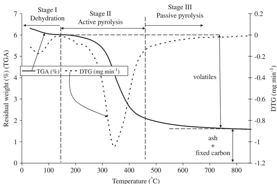
**Fig. 1 – Typical TGA diagram of corn stover in a nitrogen atmosphere.****Table 3 – Temperature range and weight loss in a nitrogen atmosphere**
