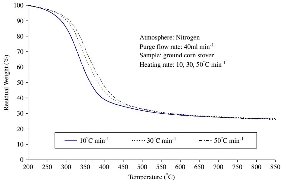
Fig. 3 – Effect of heating rates on TGA plot of corn stover in a nitrogen atmosphere.
