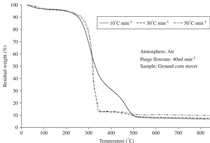
Fig. 5 – Effect of heating rates on thermogravimetric plot of corn stover in an air atmosphere.
