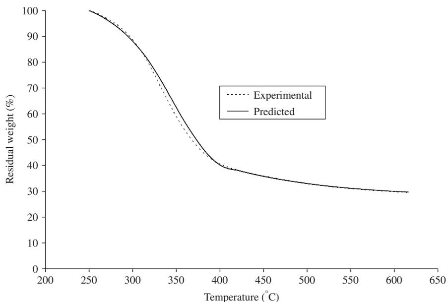
Fig. 2 – Experimental versus predicted weight loss in the temperature range of 250–800 °C, assuming two separate stages of weight loss.
