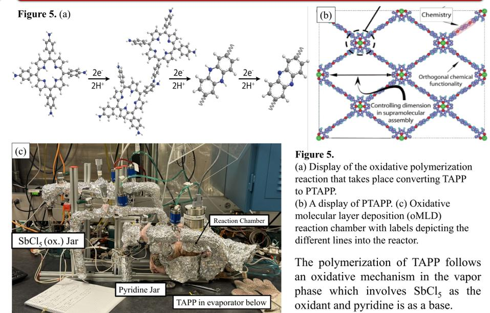
**Figure 5.** (a) Display of the oxidative polymerization reaction that takes place converting TAPP to PTAPP. (b) A display of PTAPP. (c) Oxidative molecular layer deposition (oMLD) reaction chamber with labels depicting the different lines into the reactor. The polymerization of TAPP follows an oxidative mechanism in the vapor phase which involves  $SbCl_5$  as the oxidant and pyridine is as a base.
