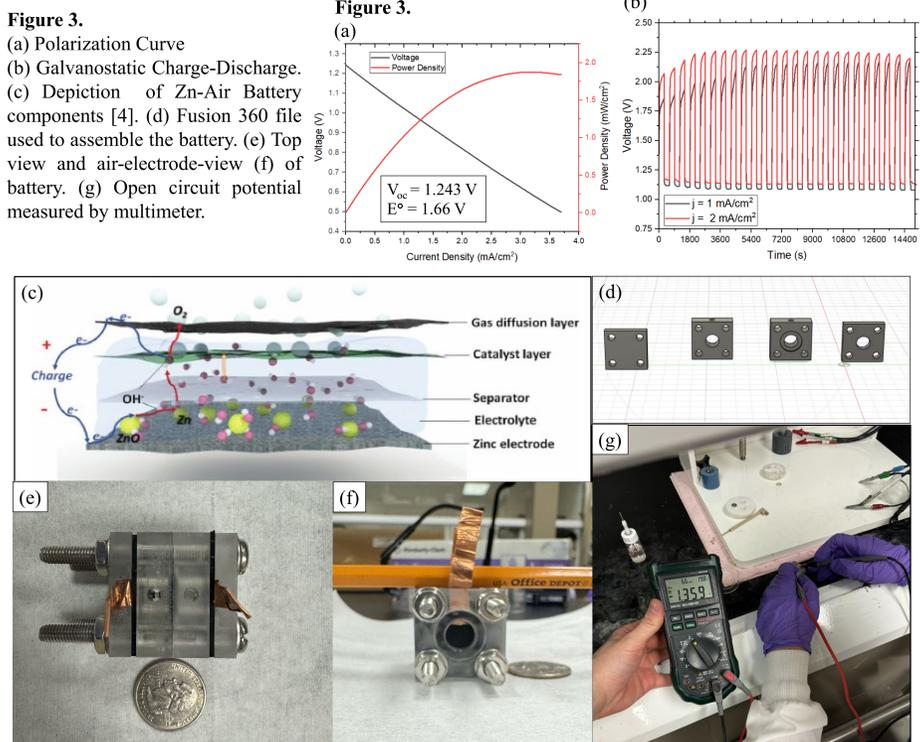
**Figure 3.** (a) Polarization Curve (b) Galvanostatic Charge-Discharge. (c) Depiction of Zn-Air Battery components [4]. (d) Fusion 360 file used to assemble the battery. (e) Top view and air-electrode-view (f) of battery. (g) Open circuit potential measured by multimeter.
