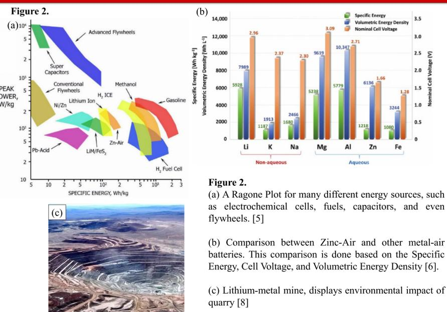
**Figure 2.** (a) A Ragone Plot for many different energy sources, such as electrochemical cells, fuels, capacitors, and even flywheels. [5] (b) Comparison between Zinc-Air and other metal-air batteries. This comparison is done based on the Specific Energy, Cell Voltage, and Volumetric Energy Density [6]. (c) Lithium-metal mine, displays environmental impact of quarry [8]
