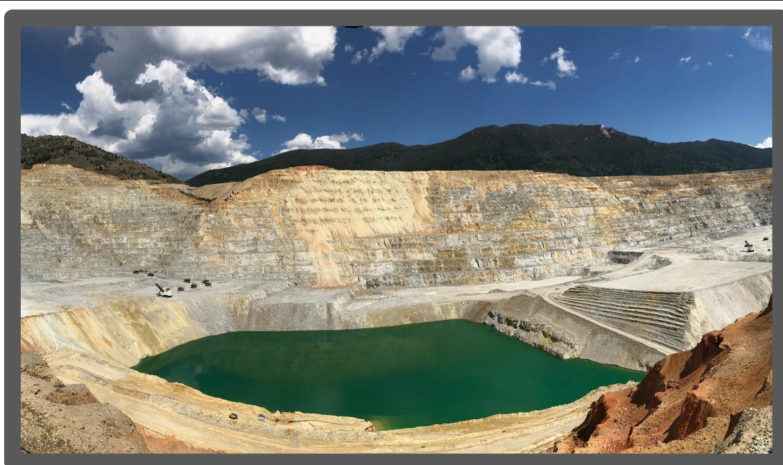
Figure 3. Berkely Pit, Butte, Montana. Mining activities that expose sulfur to rainwater create acid water drainage. This large source of undesired acidic water could serve as a source for water splitting for hydrogen production.
