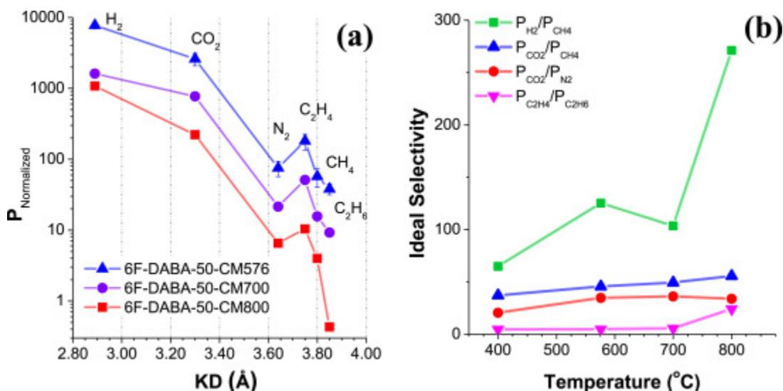
Fig. 8. 6F-DABA-50-CM membrane gas (a) permeability versus KD and (b) ideal selectivity versus pyrolysis temperature.
