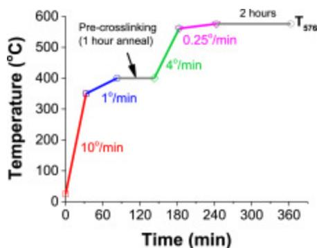
Fig. 2. Pyrolysis heating protocol for a CMS membrane formed at 576 °C.
