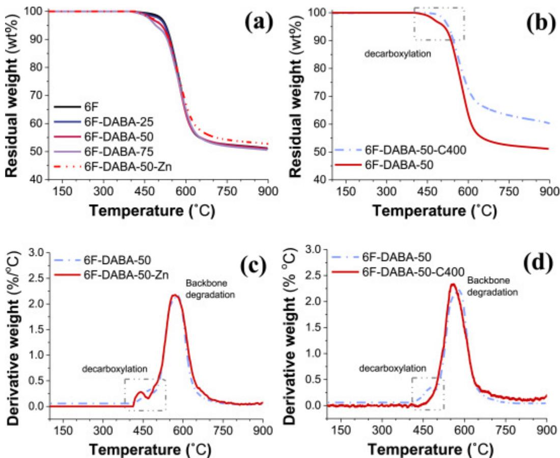
Fig. 3. TGA response for (a) 6F and 6F-DABA, (b) 6F-DABA-50 crosslinked versus non-crosslinked, (c) dynamic TGA response of derivative weight percent for 6F-DABA-50 versus 6F-DABA-50-Zn, and (d) 6F-DABA-50 crosslinked versus non-crosslinked.
