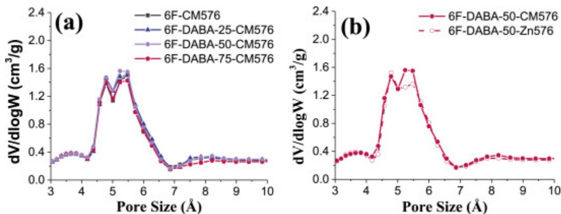
Fig. 5. CMS pore-size distribution created at 576 °C for (a) 6F and 6F-DABA series, and (b) 6F-DABA-50-CM576 versus 6F-DABA-50-Zn576.
