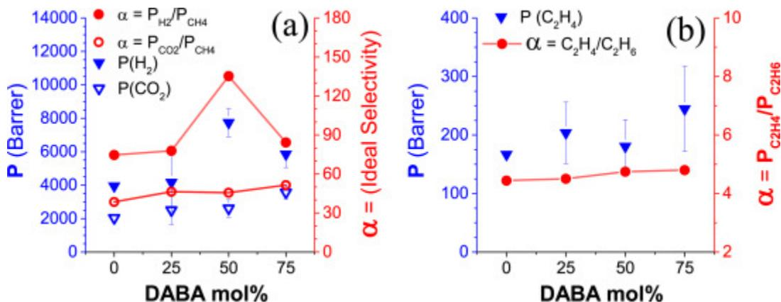
Fig. 9. CMS membranes gas permeability and ideal selectivity trend versus DABA mol% for (a) CO<sub>2</sub>/CH<sub>4</sub> and H<sub>2</sub>/CH<sub>4</sub>, and (b) C<sub>2</sub>H<sub>4</sub>/C<sub>2</sub>H<sub>6</sub>.
