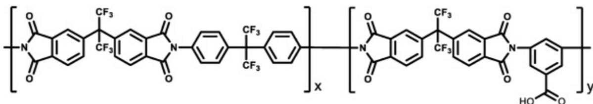
Fig. 1. Chemical structure of 6F-DABA polyimide with  $x$  and  $y$  representing 6FDA and DABA molar concentration.
