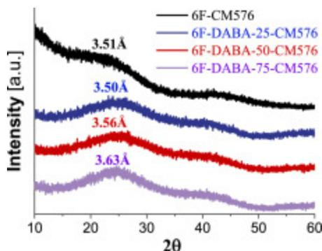
Fig. 4. Wide-angle X-ray diffraction patterns of CMS membranes derived from different polyimide precursors at 576 °C.
