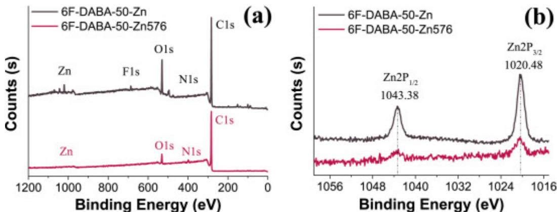
Fig. 6. 6F-DABA-50-Zn and 6F-DABA-50-Zn576 (a) wide scan XPS, and (b) XPS spectra showing  $Zn\ 2p_{3/2}$  and  $Zn\ 2p_{1/2}$  of materials.
