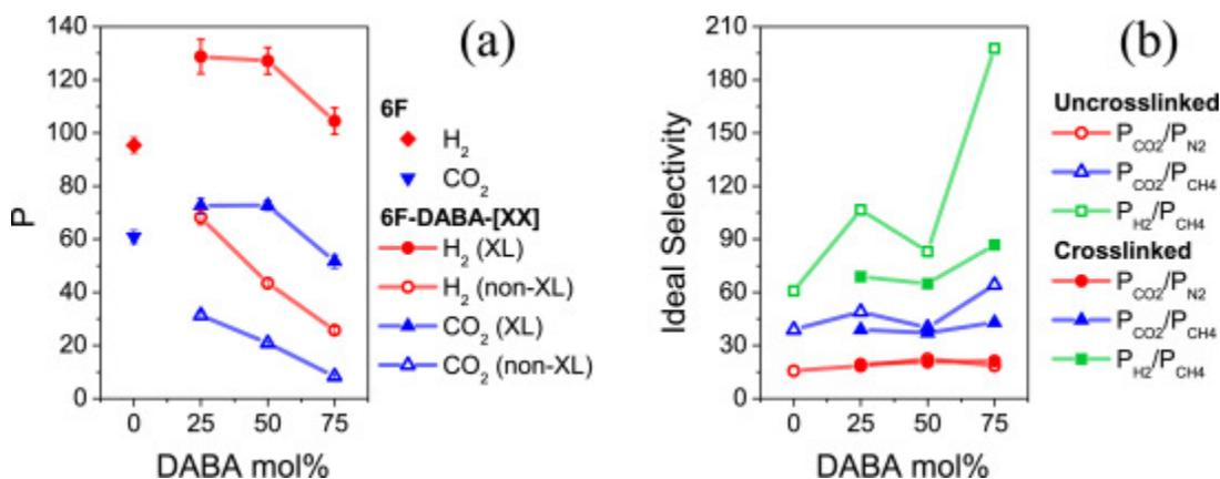
Fig. 7. 6F and 6F-DABA-[XX] crosslinked (XL) and non-crosslinked (non-XL) membrane (a) permeability and (b) ideal selectivity versus DABA mol%. The value [XX] signifies the mole % within the 6F-DABA polyimide.
