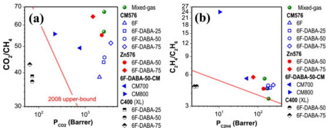
Fig. 10. CMS membrane separation comparison for (a)  $\text{CO}_2/\text{CH}_4$ , and (b)  $\text{C}_2\text{H}_4/\text{C}_2\text{H}_6$  gas pairs.
