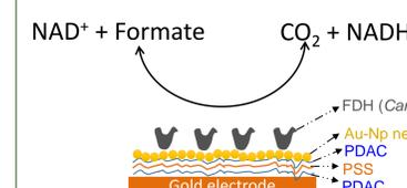
Enzyme activity assay after immobilization: the electrode with immobilized enzyme was immersed in incubation solution containing NAD<sup>+</sup> and formate.
