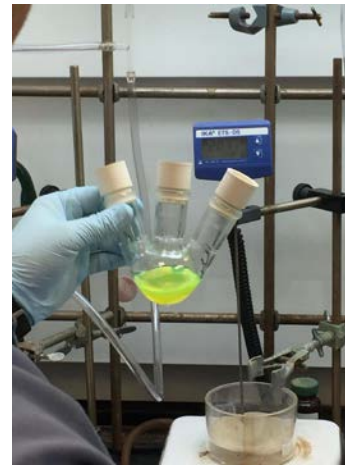
Synthesis of \text{CsPbBr}_3 Quantum Dots (QD)
