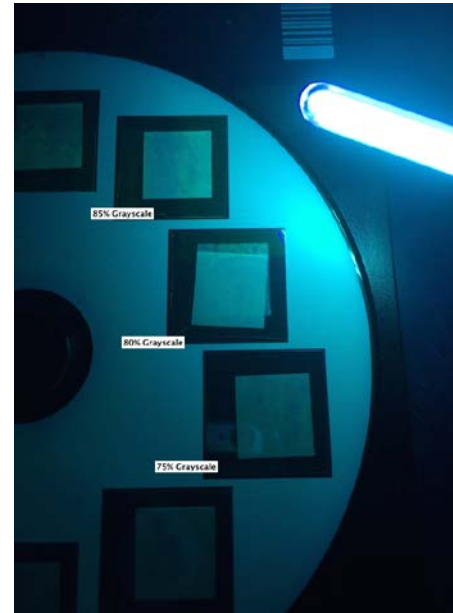
Photoluminescence of perovskite on 0% grayscale (black) to 20% grayscale (dark gray).
