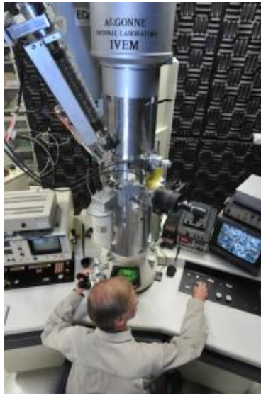
The IVEM-Tandem facility at Argonne National Lab for in situ irradiation experiment
