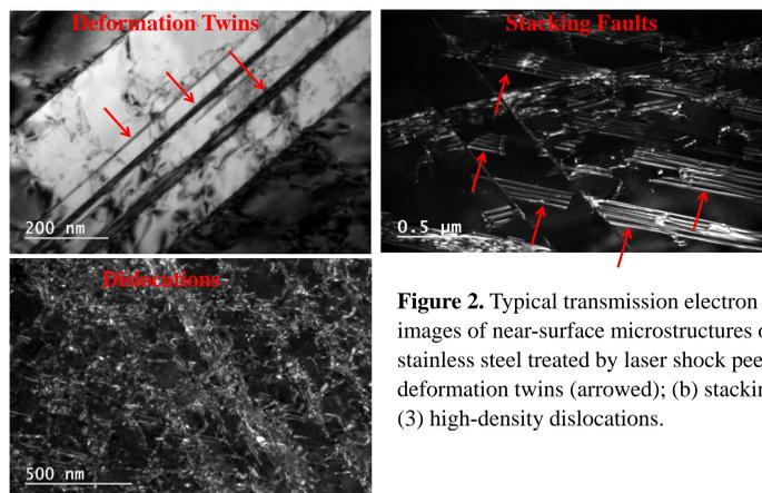
**Figure 2.** Typical transmission electron microscopy (TEM) images of near-surface microstructures of 304 austenitic stainless steel treated by laser shock peening (LSP): (a) deformation twins (arrowed); (b) stacking faults (arrowed); (3) high-density dislocations.
