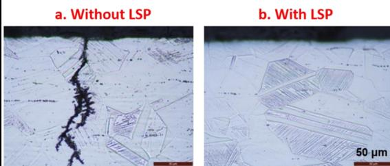
**Figure 4.** Stress corrosion cracking (SCC) test results in a hot water environment with 42% MgCl<sub>2</sub> at 144 °C for 168 hours: (a) original 304 stainless steel; (b) 304 stainless steel treated by LSP with 850 mJ laser pulse energy and 4 laser pulses. The images are optical micrographs of the cross-section microstructure.
