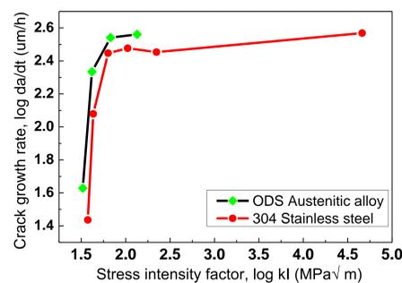
**Figure 3.** Crack growth rate diagram of the ODS austenitic alloy in comparison with 304 stainless steel.
