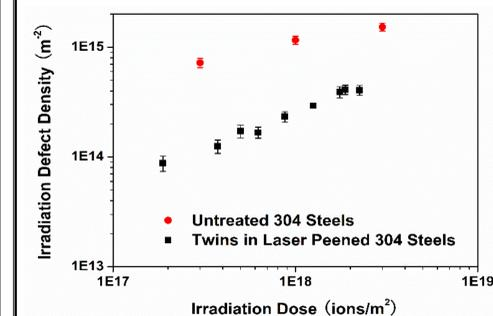
**Figure 6.** Evolution of irradiation defect density in untreated and laser-peened 304 steels (twin region) under 1 MeV Kr<sup>+</sup> irradiation at room temperature
