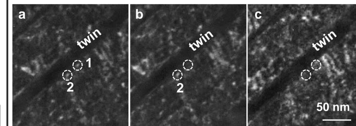
**Figure 5.** Annihilation of irradiation defects by a twin boundary in laser-peened 304 steel sample: (a) two defect clusters 1 and 2 (bright spots in circles) formed at 0s; (b) defect cluster 1 was annihilated at 4s; (c) defect cluster 2 was annihilated at 32s.
