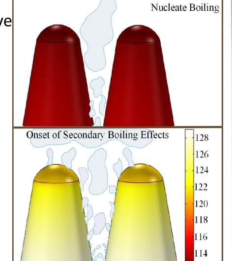
nucleation sites must be present Secondary boiling effects are due to a combination of temperature gradient (low thermal conductivity and tall microstructure height) and an wide range of potential nucleation cavities along the height of the microstructure
