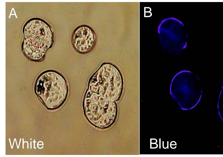
Functionalizing spheres with Resilin protein hybrids: Chitin coated agarose beads were created with recombinant Resilin fused to a protein chitin binding domain. Beads (~1mm diameter) were then treated to form Resilin cross-links by peroxidase activation, mixed with naked-untreated beads and examined by fluorescence microscopy. (A) Bright field image; (B) Blue fluorescence image; (C) Merged image.
