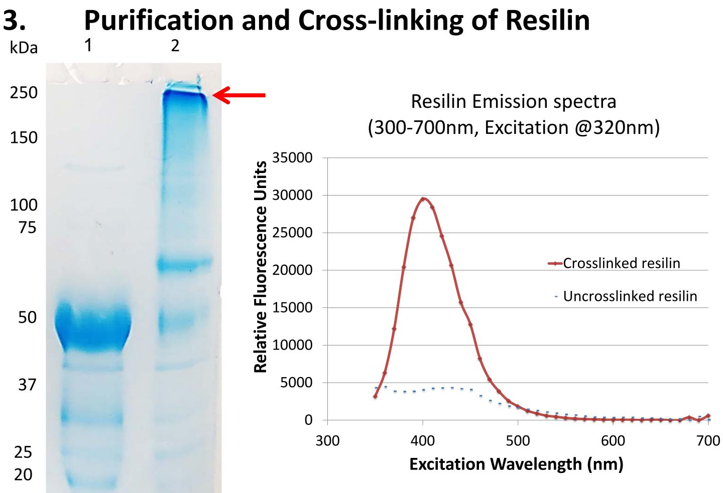
A) HRP-cross-linking: Soluble Resilin, 1 mg/mL HRP and 10 mM hydrogen peroxide, produces polymerized Resilin (arrow); lane 1, Uncross-linked Resilin; lane 2, Crosslinked Resilin (B)Fluorescence of Resilin. The fluorescence detected by scanning 300-700nm, both uncross-linked and cross-linked Resilin protein data is shown.
