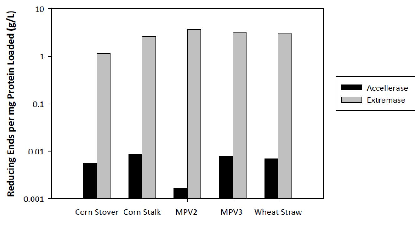
Comparison of Extremase cocktail to Accellerase 1500 cocktail. Pretreated lignocellulosic substrates were incubated with equal volumes of each cocktail at pH 3.0 and 80 C for 24 hours. Reducing ends were assayed by DNS assay at 540 nm with normalization to substrate-only controls.
