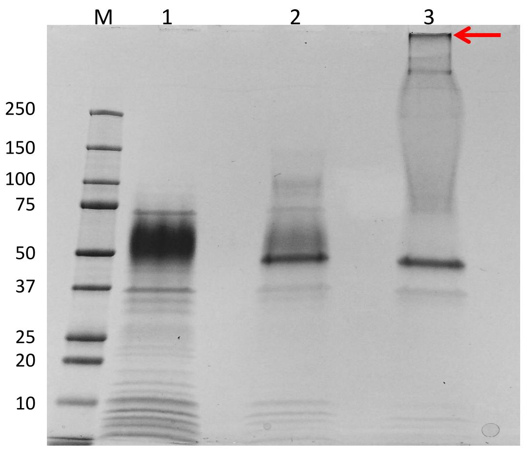
Lane 1, Heat fractionated Resilin protein (1 mg); Lane 2, Resilin HRP mixture without  $H_2O_2$ ; Lane 3, Resilin HRP mixture with  $H_2O_2$ . The solution containing 50 mg/mL heat fractionated Resilin, 1 mg/mL HRP, and 10 mM hydrogen peroxide produces polymerized Resilin after cross linking, barely enters the gel (arrow).
