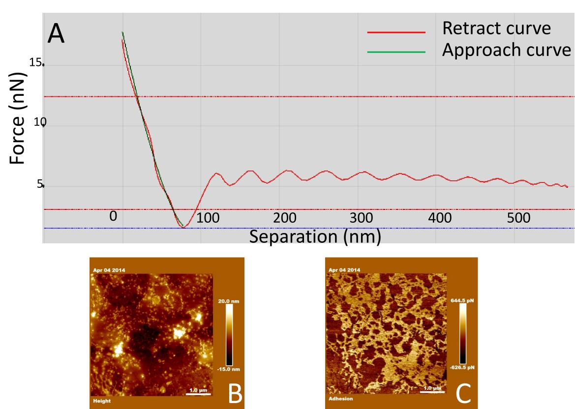
Elasticity of HRP-H<sub>2</sub>O<sub>2</sub> cross-linked Resilin by AFM : Force distance curve was recorded for cross linked resilin (A). A squared area of the length of 5 um is scanned to image the resilin surface. Two images , height (B) and adhesion (C), are depicted here. In adhesion image, the lighter color shows the softer sections.
