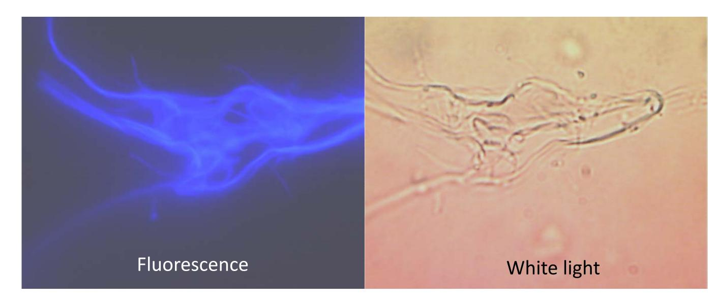
Fluorescence analysis of heat fractionated resilin sample. The pictures were taken by Nikon fluorescence microscope with a DAPI filter cube (Excitation: 358 nm)
