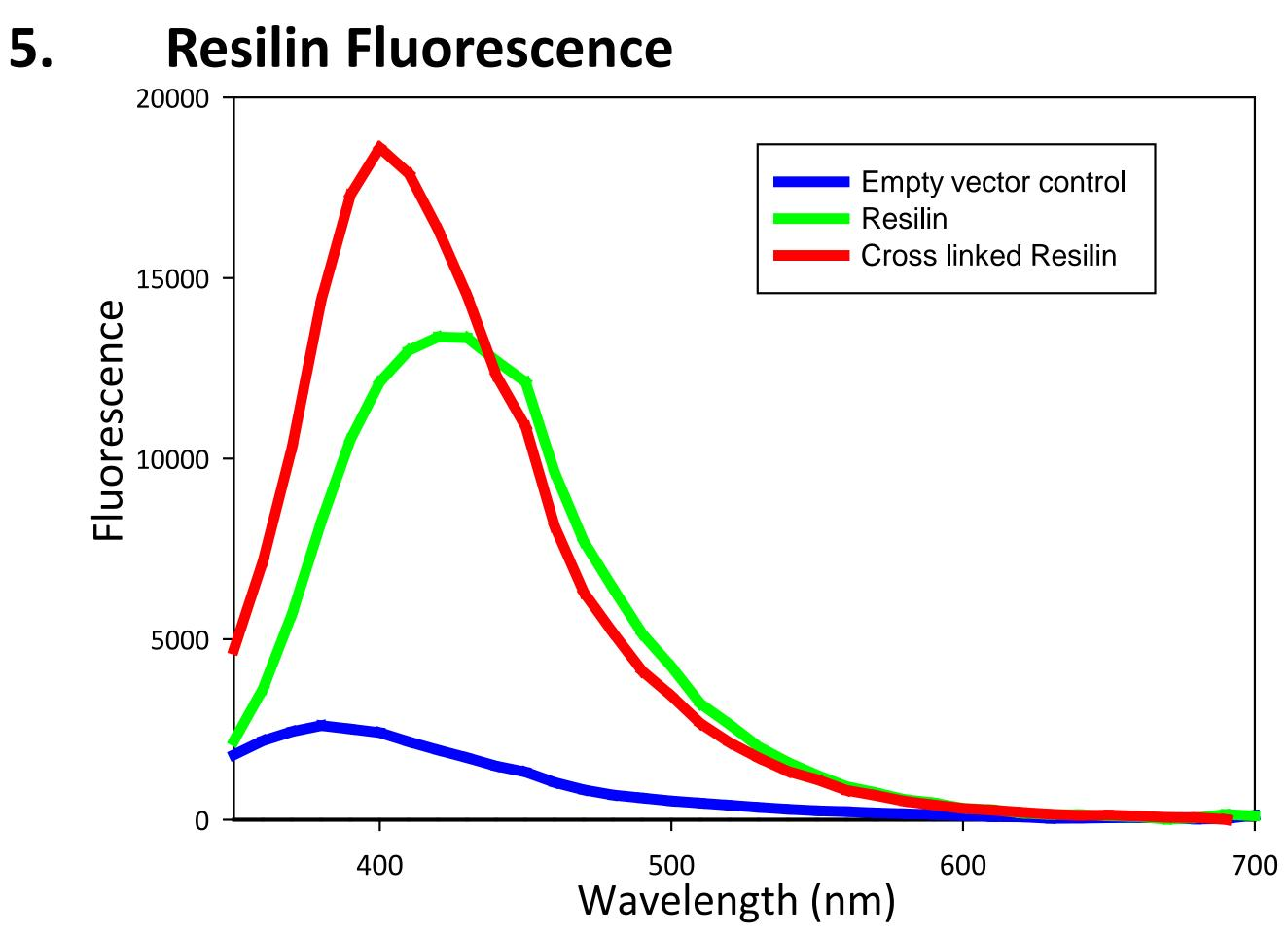
Fluorescence emission spectra of heat fractionated resilin and HRP cross linked resilin. The emission scan was from 300-700nm with excitation @ 320nm
