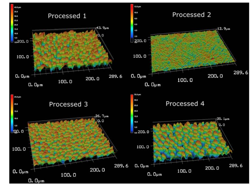
Surfaces were designed to have varying height and spacing • All surfaces were processed to be superhydrophilic (contact angle <  $5^{\circ}$ ) An additional polished (mirror finish) stainless steel surface was created for reference (not pictured)
