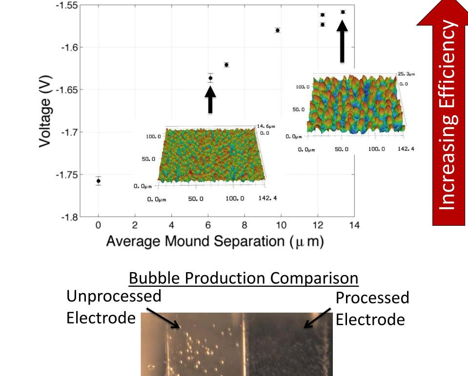
control of laser fluence and number of incident laser
