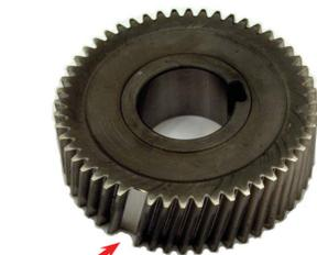
Fig. 6: The testing gear with one tooth removed.
