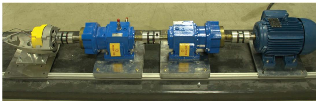
Fig. 5: The experimental system. From left to right: EXTRACTOR wind turbine, testing gearbox, speed reducer and induction machine.
