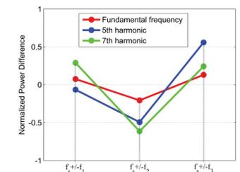
Fig. 8: Comparison of NPDs at 10% load and 297 RPM of the PM machine.
