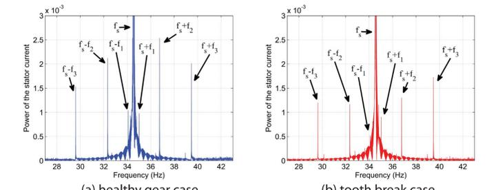
Fig. 7: Fundamental component of the stator current and its sidebands.
