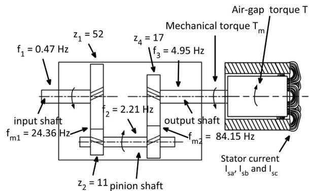
Fig. 4: Schematic of a two-stage gearbox connected to a PM machine with characteristic vibration frequencies.
