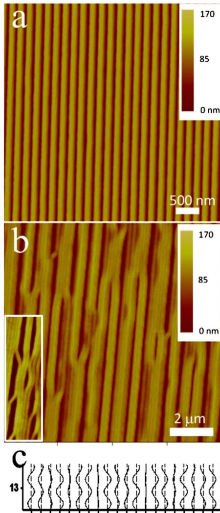
FIG. 4. (Color online) AFM topographical images of a rigid mold and fabricated PDMS structures from embossing/imprinting: (a) original mold with a pitch of 200 nm and a depth of 150 nm and (b) collective lateral buckling features, which follows mode 13 in (c). The scalar bars are 500 nm and 2  $\mu\text{m}$  in (a) and (b), respectively.
