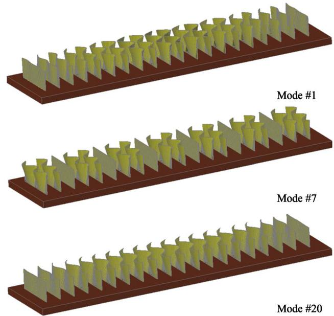
FIG. 3. (Color online) 3D structures of selected buckling modes. Top panel: mode 1, two neighboring lines buckle in opposite directions, toward or away from each other; middle panel: mode 7, several lines are not buckled; and bottom panel: mode 20, all lines buckle in the same direction.
