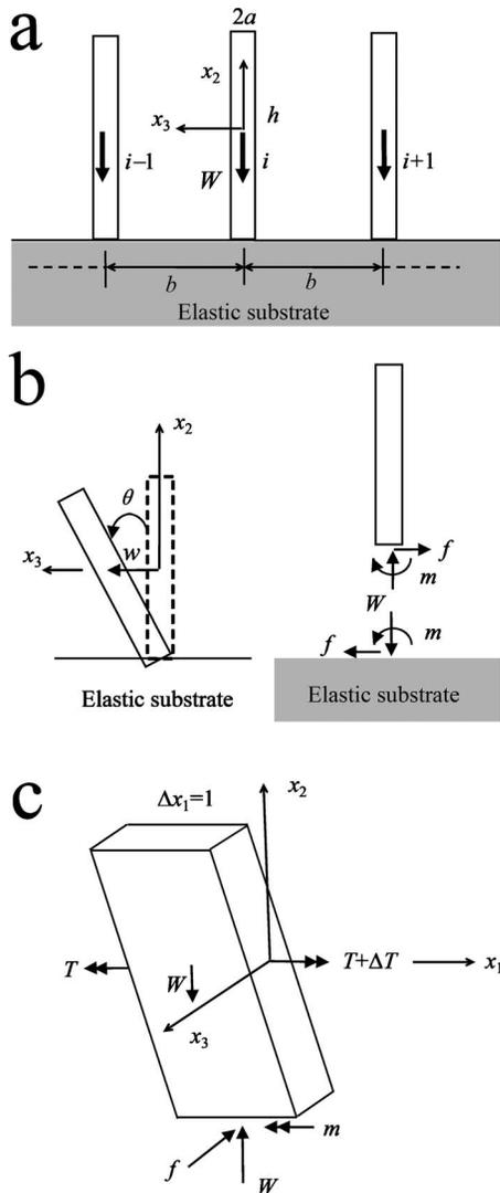
FIG. 1. Schemes for the mechanics modeling. (a) Cross section of an array of elastic lines on an elastic substrate ( $h \gg 2a$ ), (b) deflection  $w$  and rotation angle  $\theta$  of the cross section of a typical line as well as its interactions with the substrate, and (c) free body diagram for torsion of a differential element of a typical line structure.
