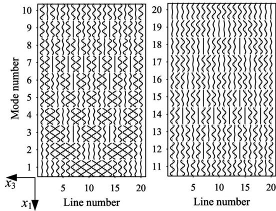
FIG. 2. Calculated modes of collective buckling on soft surface, ranked by the increasing magnitude of eigenvalues. All 20 modes are shown in this figure.
