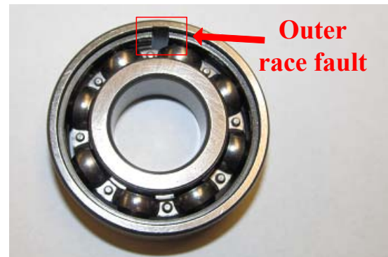
Fig. 4. The testing bearing with an outer-race fault.
