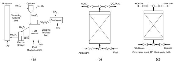
**Figure 1.** Reactor configurations for CLT: (a) Schematic of the CLC system, (b) Periodically operated CLT in packed bed system; (c)  $CO_2$  conversion to formic acid in periodically operated CLT in packed bed system.
