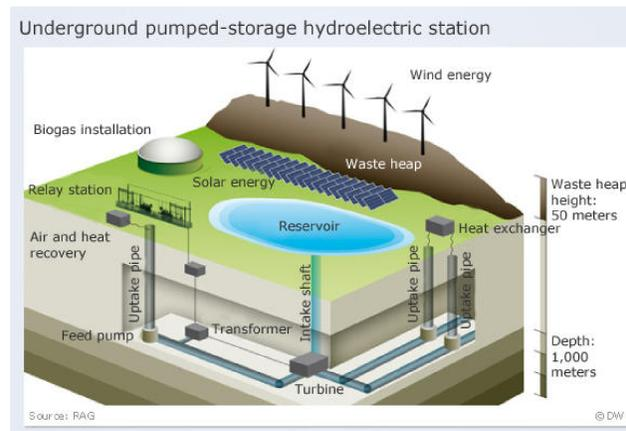
An UPHES facility has the same operating principle as PHES system: two reservoirs with a large hydraulic head between them. The only major difference between the two designs is the locations of their respective reservoirs. In conventional PHES, suitable geological formations must be identified to build the facility. However, UPHES facilities have been designed with the upper reservoir at ground level and the lower reservoir deep below the earth's surface [2].
