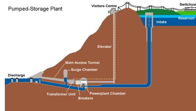
PHES is the most mature and largest storage technique available and consists of two large reservoirs located at different elevations and a number of pump/turbine units. During off-peak electrical demand, water is pumped from the lower reservoir to the higher reservoir where it is stored until it is needed. Once required the water in the upper reservoir is released through the turbines, which are connected to generators that produce electricity [2].
