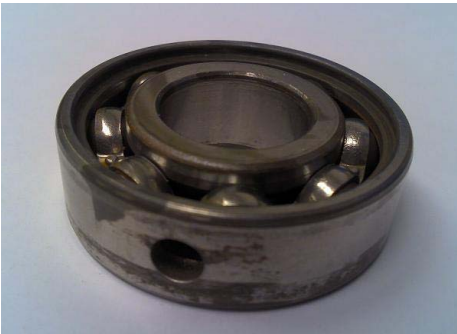
Fig. 10. The testing bearing with an outer-race fault.
