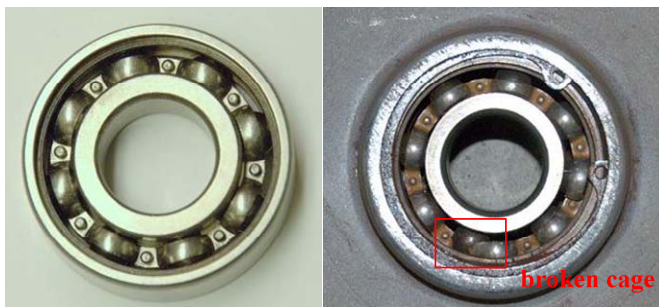
Fig. 6. The testing bearing before and after the experiment.
