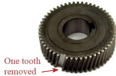
Fig. 4. The testing gear with one tooth removed.
