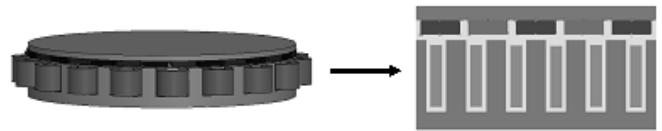
Fig. 1. Illustration of the 2D modeling of an AFPM machine.
