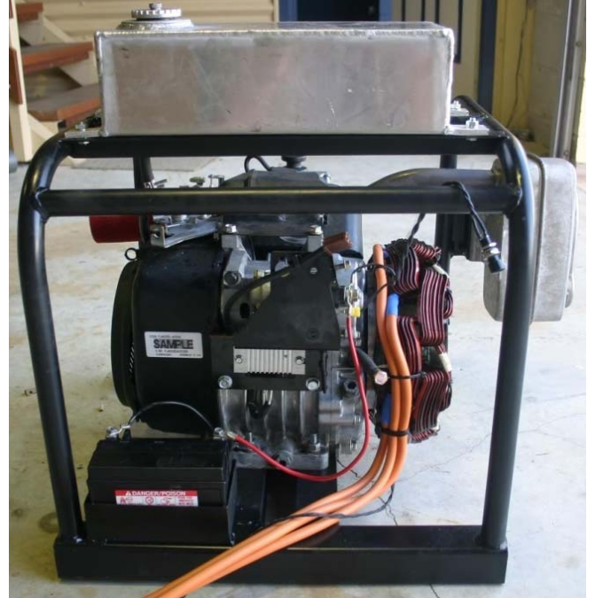
Fig. 1: 11 hp (8kW) i.c. engine with 8kW single sided axial flux starter alternator attached
