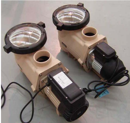
Fig. 4. Pump assemblies, with the original single phase induction machine version on left, PM axial flux version on right
