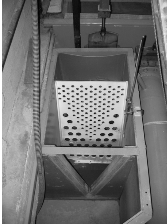
Figure 3.7 The V-Notch weir used to measure discharges in the lab.
