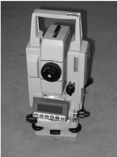
Figure 3.3 Sokkia total station
