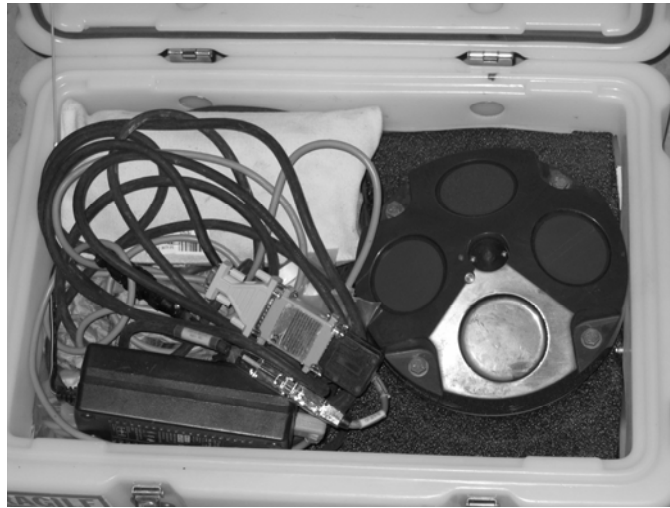
Figure 3.8 Workhorse Rio Grande 1200 kHz ADCP
