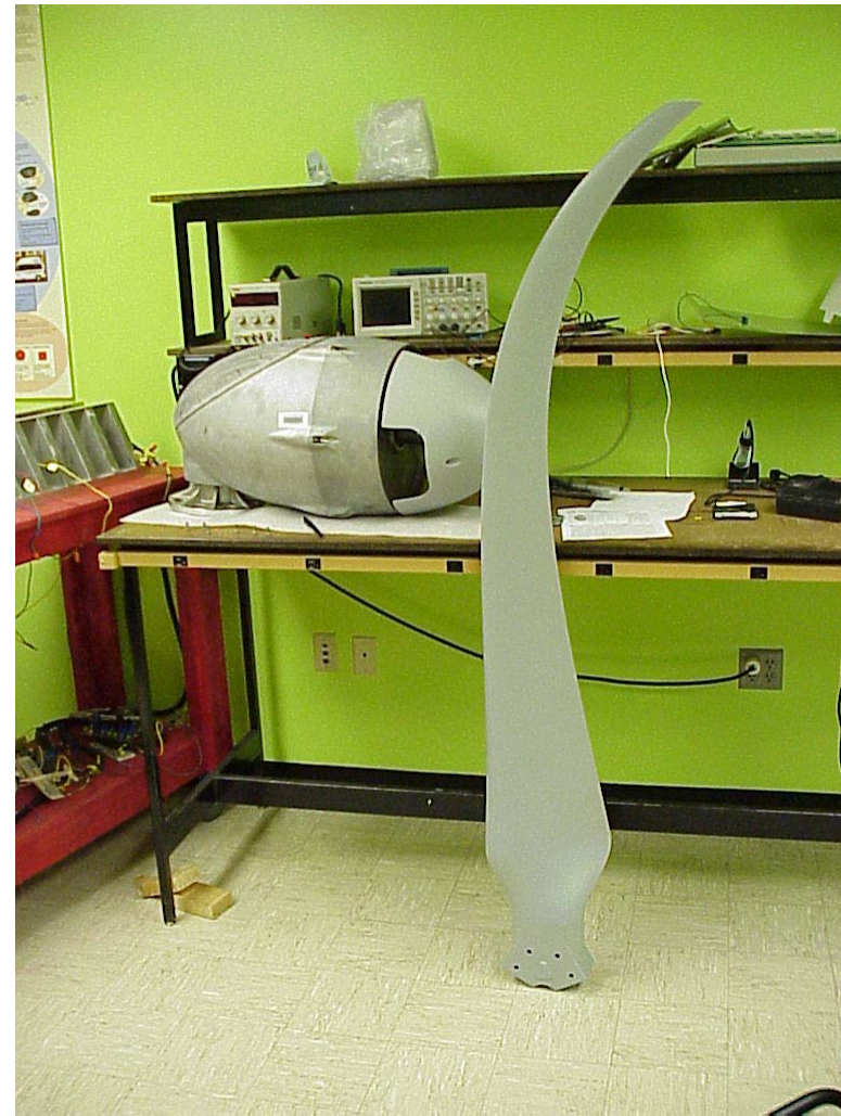
Shown: nacelle and single blade
